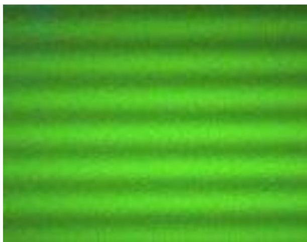
Figure 3. A fluorescence gradient/fringe pattern picture of an FITC sample. The interfringe distance corresponds to 17 \mu\text{m} .
