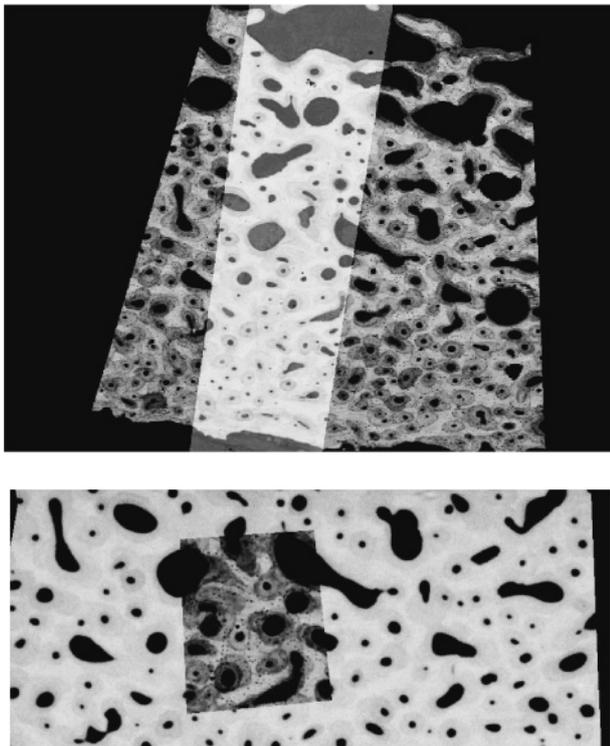
**Fig. 1.** SAM image before nanoindentation fused with SAM image after nanoindentation (up) and SR- $\mu$ CT image fused with SAM image after nanoindentation (down).
