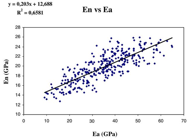
**Fig. 3.** (Color online) Correlation curve between  $E_a$  measured by acoustic microscopy and  $E_n$  derived from nanoindentation.
