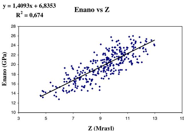
**Fig. 2.** (Color online) Correlation curve between Z measured by acoustic microscopy and  $E_n$  derived from nanoindentation.
