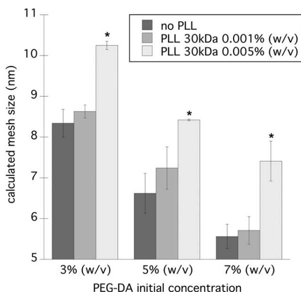
**Figure 3.** Mesh size calculations for three hydrogel formulations with different adhesive properties ( $n = 3$  for each formulation). \* $P < 0.05$  versus PEG-DA concentrations (3, 5, and 7%) with no PLL.
