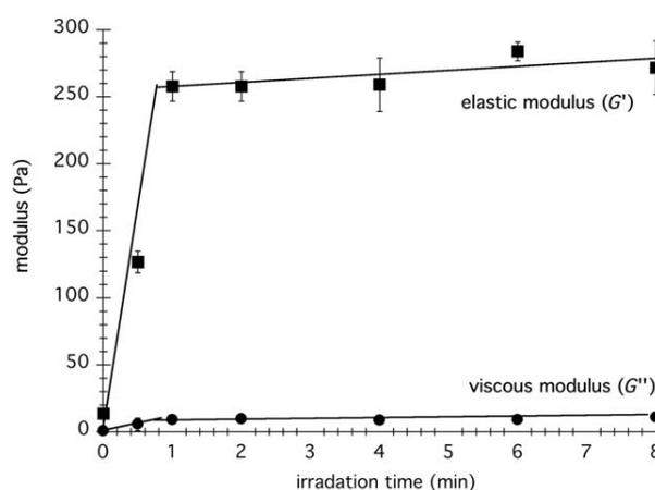
**Figure 4.** Time course of the photopolymerization of a PEG-DA 6kDa 3% w/v precursor solution, showing  $G'$  (elastic contribution) and  $G''$  (viscous contribution) moduli versus UV ( $\lambda = 365$  nm) irradiation times.
