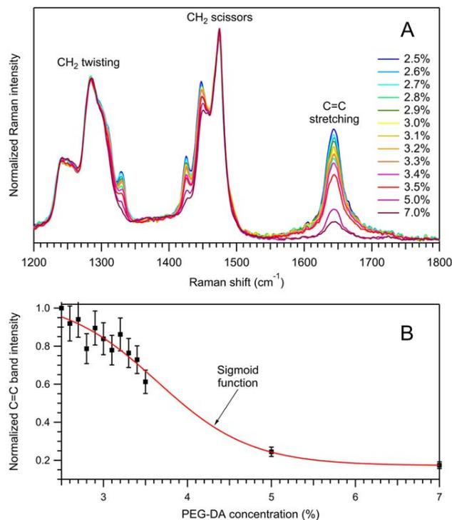
**Figure 2.** (a) Raman spectral fingerprints of PEG-DA hydrogels recorded at various hydrogels concentrations probed. Raman spectra were normalized on H—C—H deformation modes at  $1285\text{ cm}^{-1}$  ( $\text{CH}_2$  twisting) and  $1475\text{ cm}^{-1}$  ( $\text{CH}_2$  scissors). (b) Normalized C=C band intensity integrated within  $1600\text{--}1690\text{ cm}^{-1}$  range as a function of PEG-DA concentration. [Color figure can be viewed at wileyonlinelibrary.com]
