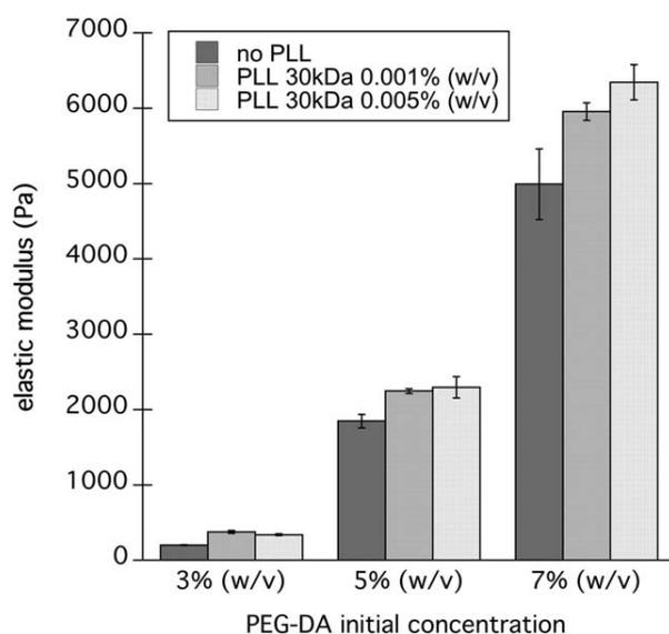
**Figure 5.** Elastic modulus representing mechanical properties of different hydrogel formulations (PEG-DA 6 kDa, with or without PLL-A 30 kDa) with variable adhesive properties ( $n = 3$  for each hydrogel condition).
