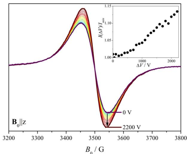
**Figure 3.** X-band EPR single-crystal data of **1** at  $B_0 \parallel z$  under varying electric fields. Experimental conditions:  $f = 9.80$  GHz, mod. ampl. =  $10 G_{pp}$ , power:  $2$  mW. The inset shows the electric field dependence of the integrated intensities of the experimental spectra ( $I_{min} = 1$ ).
