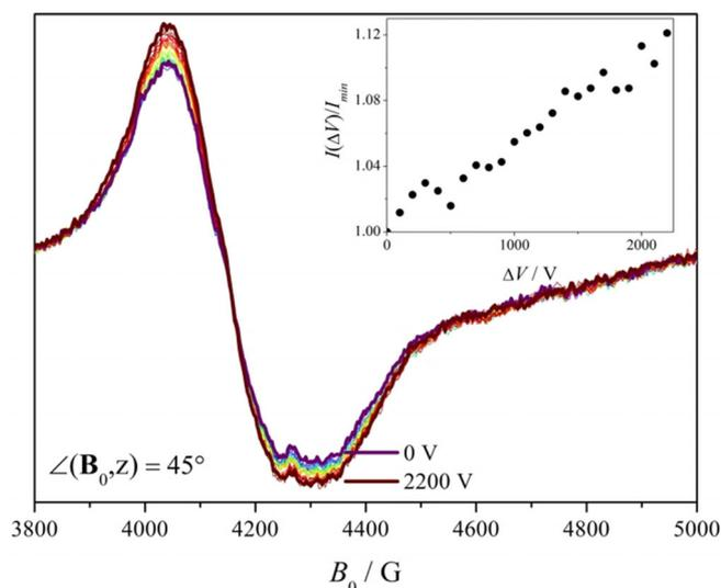
**Figure 4.** X-band EPR single crystal data of **1** at  $\angle(\mathbf{B}_0, \mathbf{z}) = \pi/4$  under varying electric fields. Experimental conditions:  $f = 9.80$  GHz, mod. ampl. =  $10 G_{\text{ppr}}$ , power: 4 mW. The inset shows the electric field dependence of the integrated intensities of the experimental spectra ( $I_{\min} = 1$ ).
