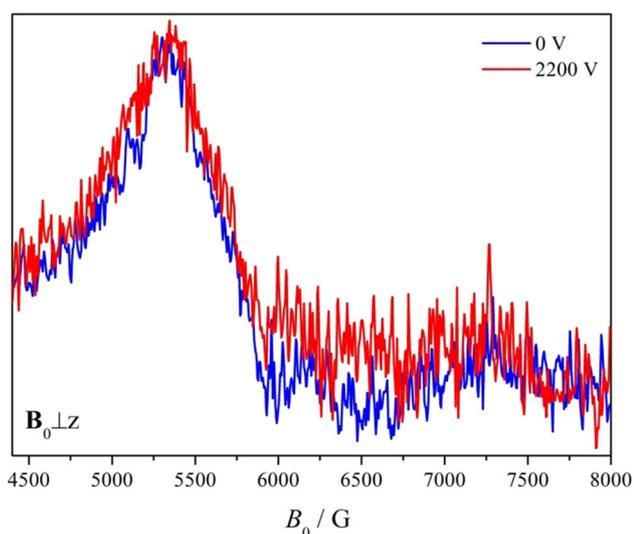
**Figure 5.** X-band EPR single crystal data of **1** at  $\mathbf{B}_0 \perp \mathbf{z}$  inside and outside an electric field. Experimental conditions:  $f = 9.80$  GHz, mod. ampl. =  $15 G_{\text{ppr}}$ , power: 6.2 mW.
