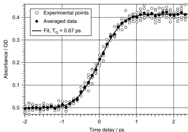
**Figure 4.** Determination of the zero-delay time point and instrumental response function via photoinduced absorption changes in copper(II)-octaethylporphyrin in toluene (2-mm path length cell). The pump and probe pulses were those used in TR<sup>3</sup> experiment without any change in energy, wavelength, or optical path. Open markers are the measured data points (five scans), filled markers are the averaged data points, and the solid curve represents the fit using Eqn (1).
