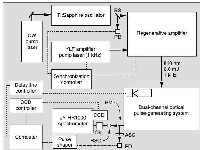
**Figure 1.** Overview of the system for sub-picosecond Raman measurements. The solid line between blocks is the laser beam, while the dashed line represents an electronic signal. PD, photodiode; BS, beam-splitter; Obj, objective; RM, retractable mirror; ASC, absorption sample cell; RSC, Raman sample cell. The specially designed dual-channel optical pulse-generating system is detailed in Fig. 2.
