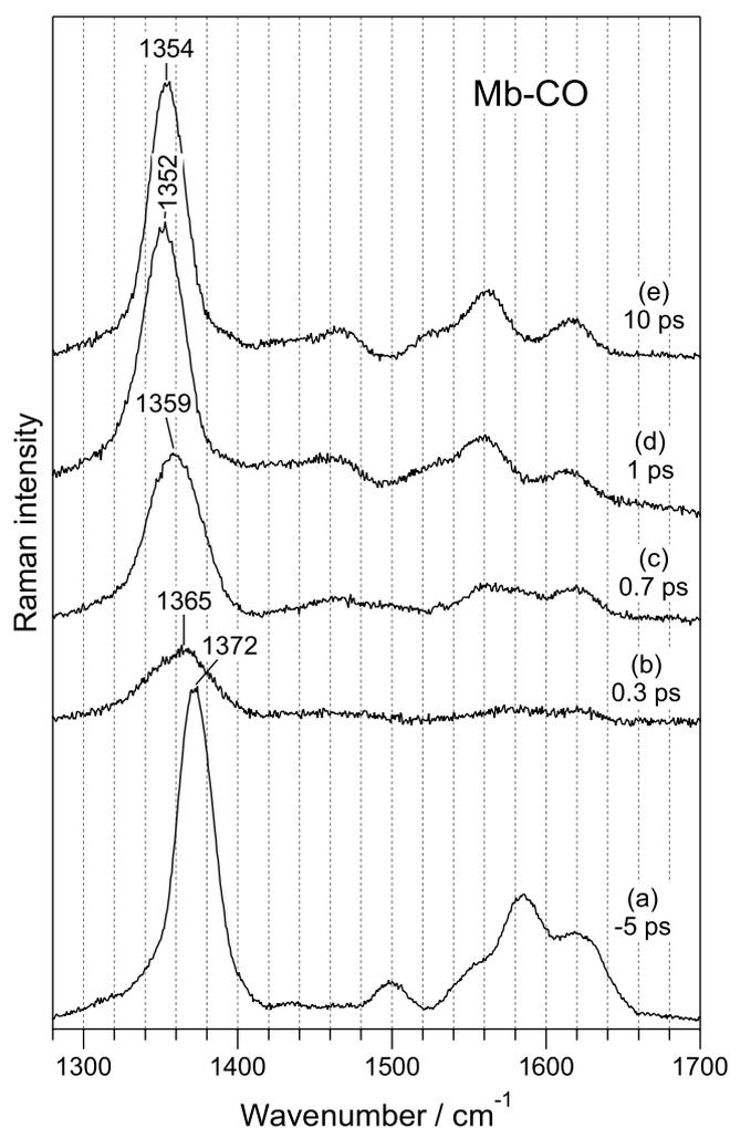
**Figure 7.** TR<sup>3</sup> spectra in the high wavenumber range of the Mb-CO complex ( $\lambda_{\text{pump}} = 570 \text{ nm}$ ,  $\lambda_{\text{probe}} = 435 \text{ nm}$ , accumulation time = 10 min). Spectrum (a) represents the ground-state Mb-CO, while the difference spectra (b-e) correspond to the Mb photoproduct at  $\Delta t = 0.3 \text{ ps}$  (b), 0.7 ps (c), 1 ps (d), and 10 ps (e).
